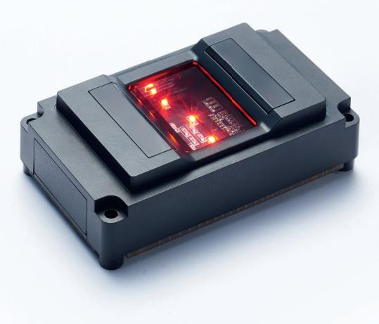
SFU-S20A is a FBI and Mobile ID FAP20 certified fingerprint scanner module that provides a number of industry-leading features under its sleek design. Featuring range-leading powerful 1.0GHz CPU, SFU-S20A provides high-speed extraction and matching of fingerprints within the scanner. SFU-S20A also supports true plug-n-play by featuring HID(human interface device) protocol. SFU-S20A is a versatile identification solution for both public and civil ID applications.
