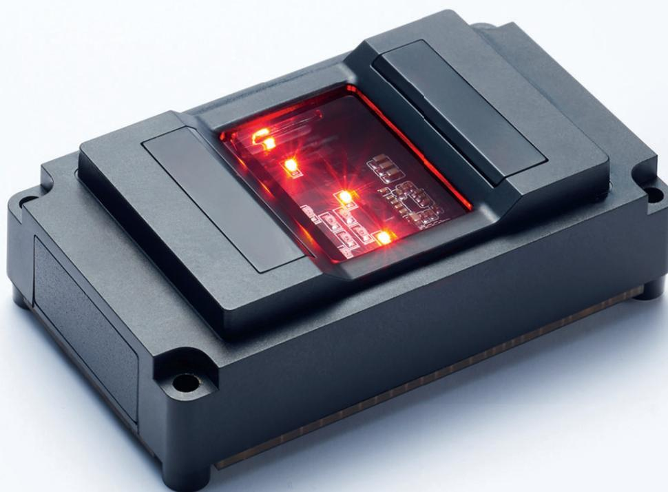
SFU-S20A is a FBI and Mobile ID FAP20 certified fingerprint scanner module that provides a number of industry-leading features under its sleek design. Featuring range-leading powerful 1.0GHz CPU, SFU-S20A provides high-speed extraction and matching of fingerprints within the scanner. SFU-S20A also supports true plug-n-play by featuring HID(human interface device) protocol. SFU-S20A is a versatile identification solution for both public and civil ID applications.
