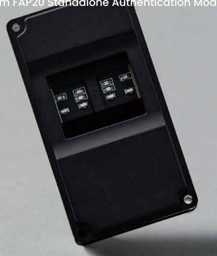
BM-Slim2S is a FBI PIV and Mobile ID FAP20 certified fingerprint module that provides a number of industry-leading features under its sleek design. Featuring range-leading powerful 1.0GHz CPU, BM-Slim 2S provides high-speed extraction and matching of fingerprints within the scanner.
